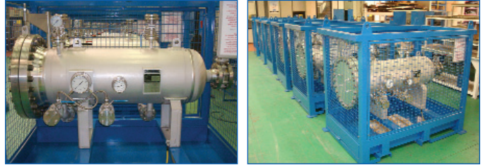
4S Simplex High Flow filter rental skid
